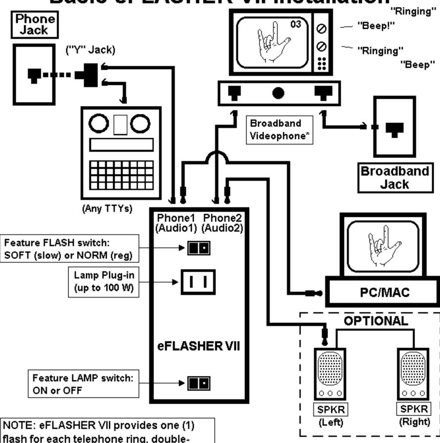
NOTE: eFLASHER VII provides one (1) flash for each telephone ring, doubleflashes (2) for each Broadband ring, and three flashes (3) for each computer call. For computer call, a sound .WAV file must be used to operate which it can be download from manufacturer's website: http://www.deafworks.com/eFLASHER/download.html
