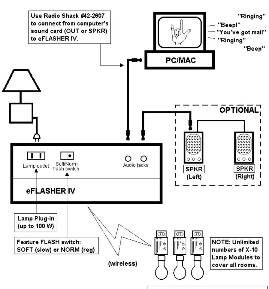
NOTE: eFLASHER IV provides three (3) flashes for each computer sound or call signal received. Must use a special .WAV file to operate it which it can be download from manufacturer's website:
