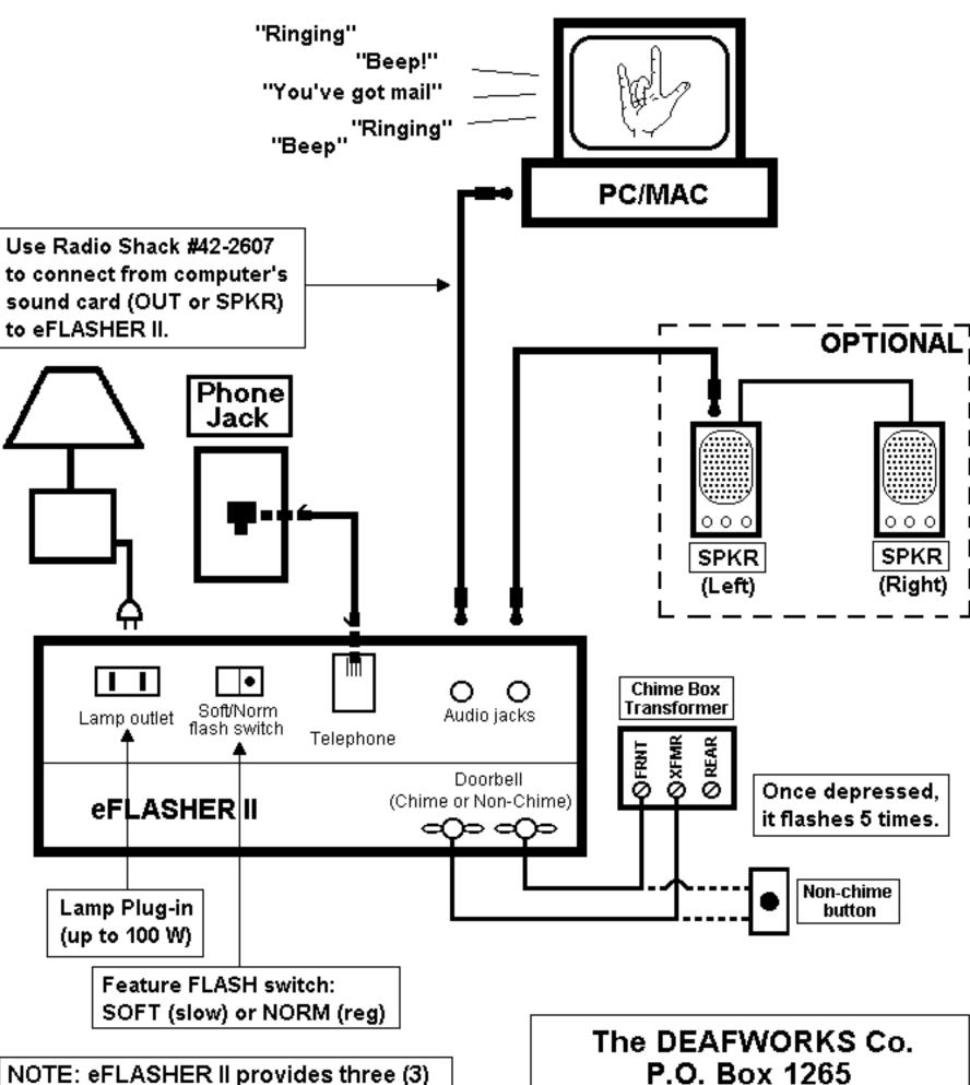
NOTE: eFLASHER II provides three (3) flashes for each computer sound or call signal received. Must use a special .WAV file to operate it which it can be download from manufacturer's website:
